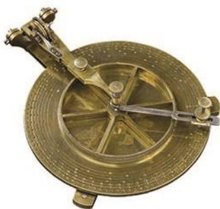
Instrument for ruling clock dials
