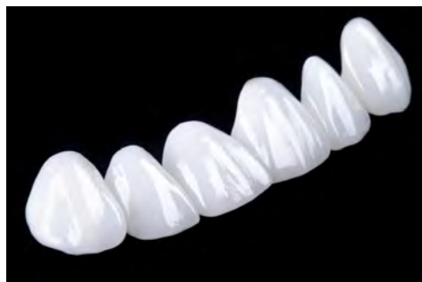
▲ Zirconia is a very strong and biocompatible advanced ceramic material. Zirconia tooth crowns are used to replace missing teeth.
