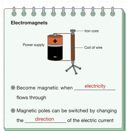
Maglev trains make use of electromagnets to levitate and move. Experience the exhibit "When the current flows, things are magnetised". What can you observe?
