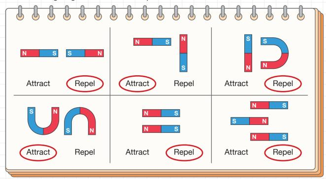
Maglev trains make use of the repulsive force between same pole to push the train up and levitate.
